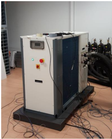
Figure 2: Picture of the reversible dual source heat pump during tests performed at Hired.
