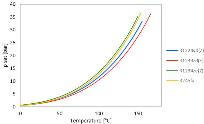
Figure 1. Fluids saturation pressure according to RefProp v.10.0
