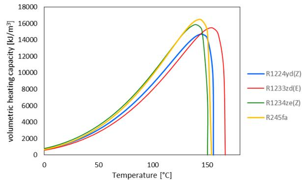
Figure 3. Volumetric heating capacity
