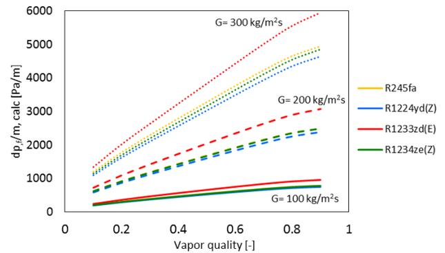
Figure 5. Frictional pressure drops during condensation at 92°C,  $x=0.5$ , according to Friedel (1979)
