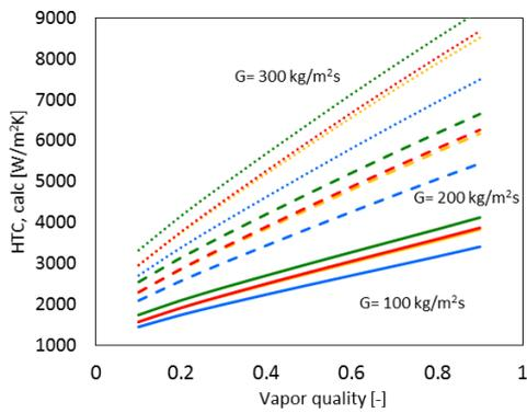
Figure 4. Condensation heat transfer coefficient at 92°C,  $x=0.5$ , according to Cavallini et al. (2006)
