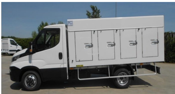
Figure 8: Reference body truck used in climatic chamber.
