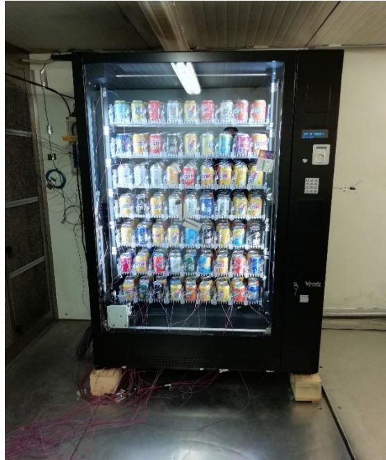
Figure 2: Vending machine in climatic chamber.
