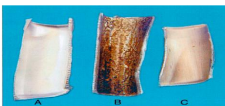
A: New evaporator tube B: Untreated evaporator tube after 400 hours of operation. C: Evaporator tube treated with additive after 400 hours of operation.
